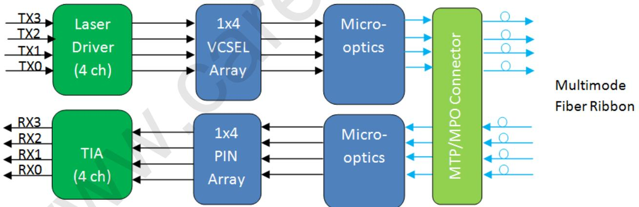
**Figure 1. 100G CFP4 SR4 Transceiver Block Diagram**
